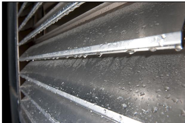
BSRIA Limited, Rain and airflow test for storm louvres according to BS EN 13030
